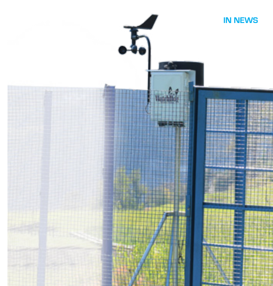
Above: The automatic weather recording station installed in Tipli village that monitors weather patterns and gives accurate data based on which scientists conclude their predictions
